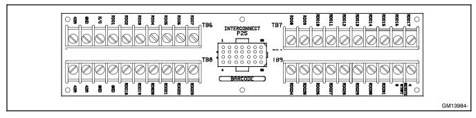
Figure 6-39 Terminal Strips TB6, TB7, TB8, and TB9 on the Controller Connection Kit in the Junction Box
